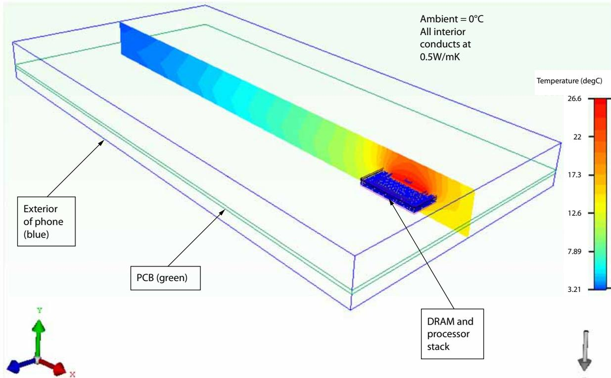
Figure 2: Cell Phone Thermal Simulation - Side View
