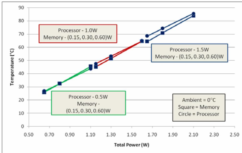
Figure 4 is a graphical illustration of power-consumption estimates for processor power (0.5W, 1.0W, and 1.5W) and memory power (0.15W, 0.30W, and 0.60W) cross-temperature.
