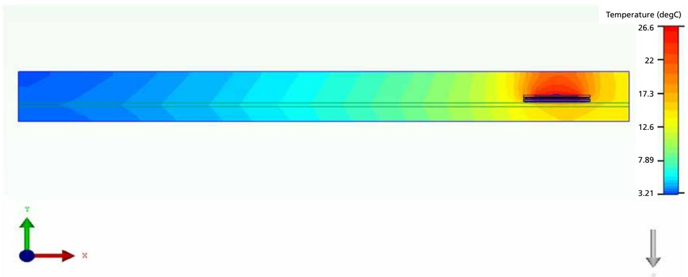
Figure 3: Cell Phone Thermal Simulation PoP Stack
