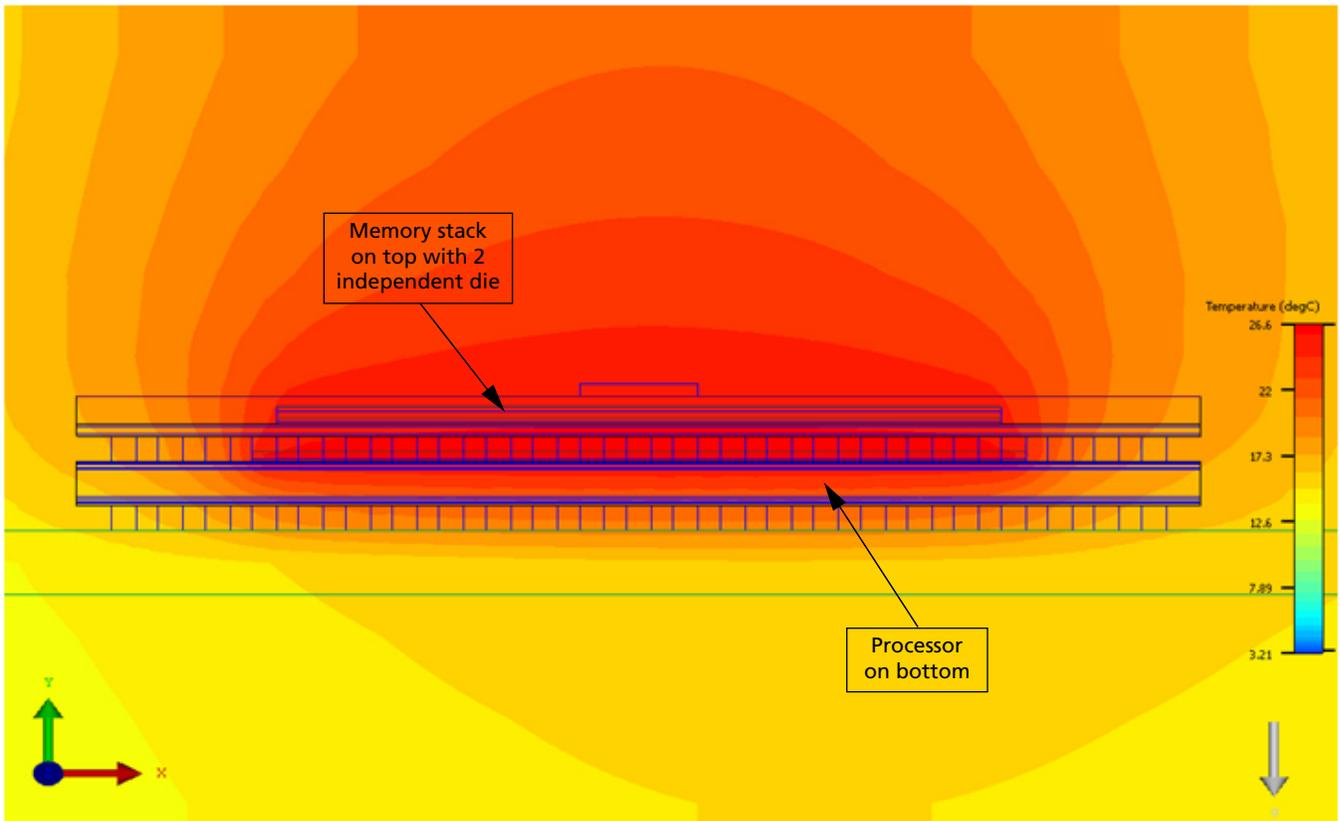
The simulation shows that the processor and memory stack will operate at very close to the same temperatures.
