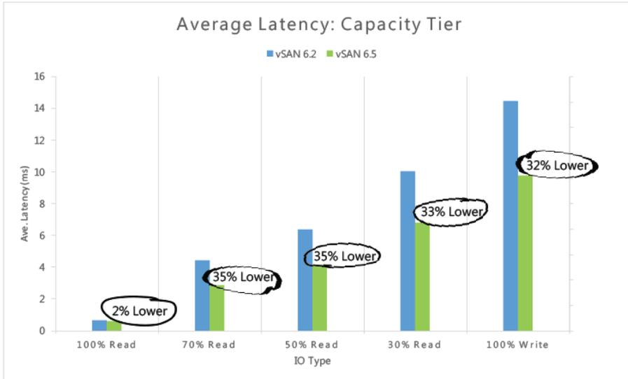
**Figure 2b: Capacity Tier Average Latency**
