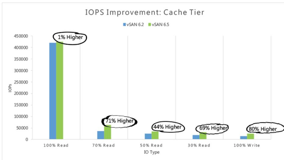
Figure 1a shows the IOPS difference across the five measured IO profiles.
