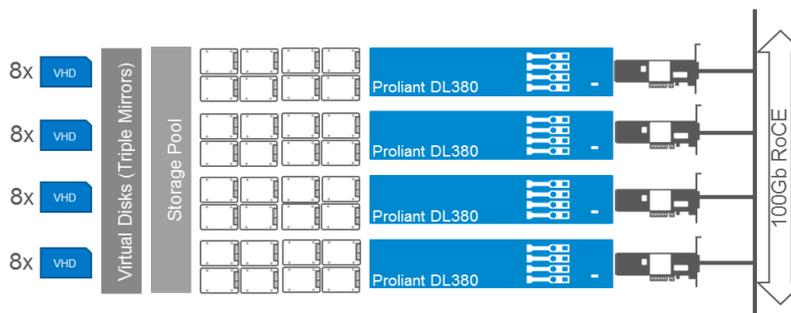
Figure 5: Single-Tier Hyper-V With S2D Test Configuration
