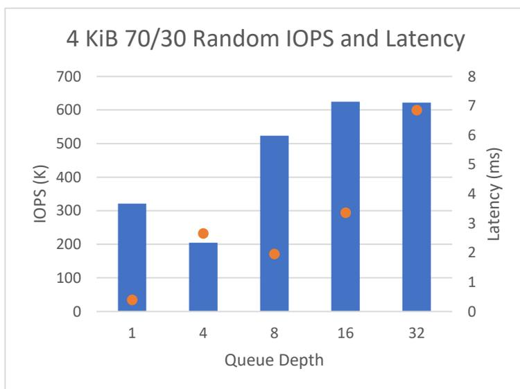
Figure 2: Low-Latency Random I/O for Mixed Read/Write Workloads
