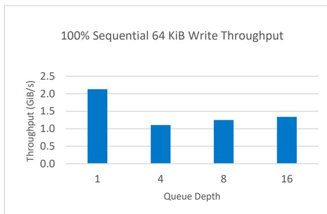
Figure 4: 100% Write Throughput Results
