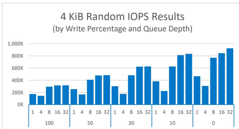
Figure 1: Micron SATA All-Flash S2D 4 KiB Random IO Results
