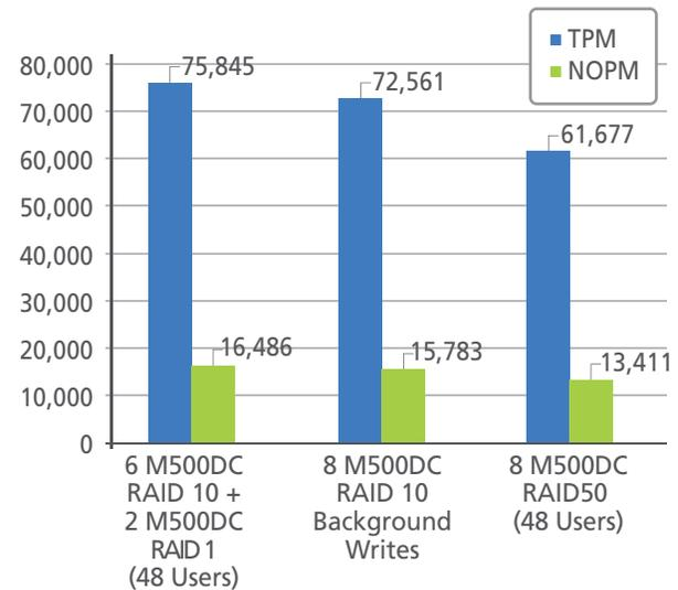
**Figure 3: Effect of RAID Configuration on M500DC Performance**
