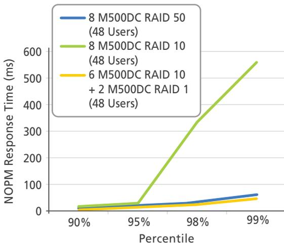
**Figure 4: Times With Different RAID Configurations**
