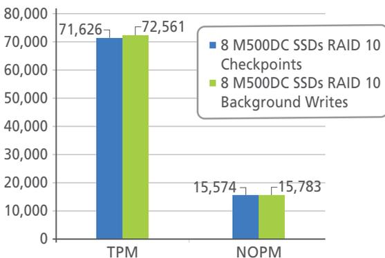
**Figure 1: Performance of 8 M500DC SSDs With Checkpoints vs. Background Writes**
