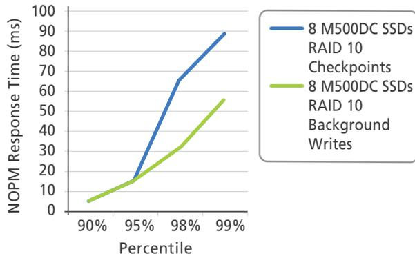
**Figure 2: Latency of 8 M500DC SSDs With Checkpoints vs. Background Writes**
