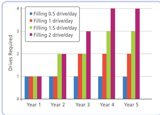
**FIGURE 1: Number of drives required for different fill rates using a one-half-fill-per-day drive**
