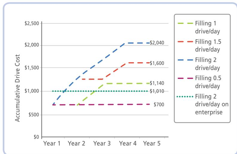
**FIGURE 2: TCO of purchasing a lower-endurance SSD and replacing it as needed vs. purchasing a high-endurance SSD**
