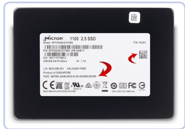
Figure 1: Micron SED with 32-Character PSID and Corresponding 2D Bar Code
