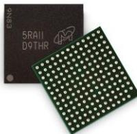
GDDR6N is a high-performance memory solution that delivers faster processing and buffering with two efficient, dual 16-bit channels and data rates up to 12 Gb/s. That's 8X the effective bandwidth of the fastest available DDR4 device. GDDR6N addresses high-performance demands, providing an alternative to standard DDR memories.
