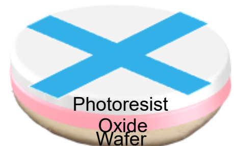
Schematic after step 3 is completed. "X" pattern represents reticle or mask.
