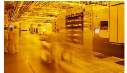
Notice the yellow light in the Photolithography area of the fab
