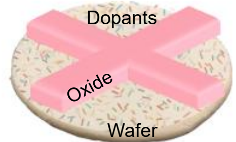
Schematic after step 7 is completed.
