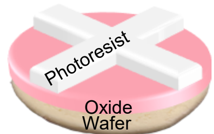
Schematic after step 4 is completed.
