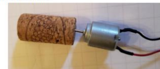
Cork centered will not create wiggling motion
