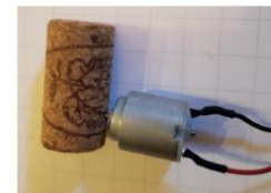
Off-centered creates wiggling motion
