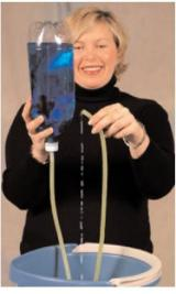
Fill the clear bottle ¾ full with water, add food coloring, and assemble it with the tubing as shown.
