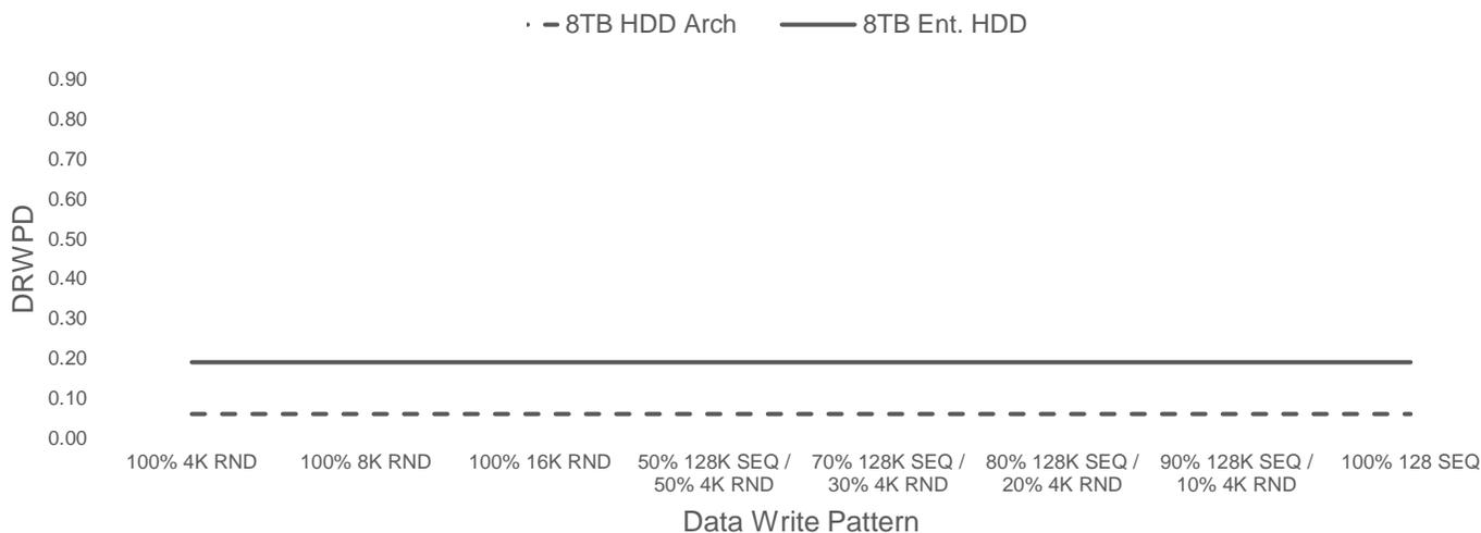
**Figure 4: HDD DRWPD by Write Pattern (workload)**
