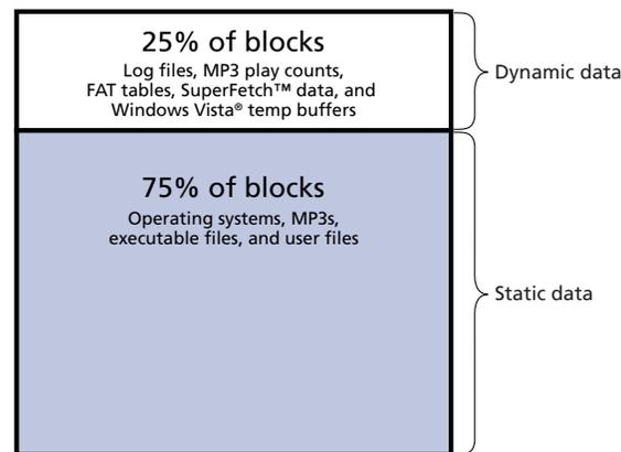
In a 4,096-block MLC device with a 10,000-cycle count, 75% static data, and a program and erase rate of 50 blocks every 10 minutes (or 6 files per hour), dynamic wear leveling results in device wear-out after approximately 4 years, with 75% of the blocks nearly unused (see Figure 3 on page 4).
