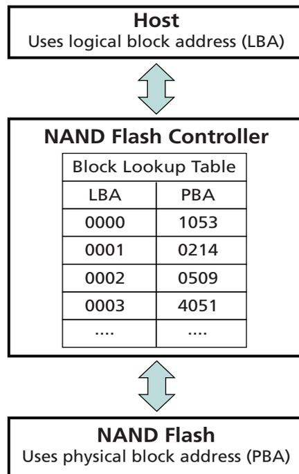
Depending on the wear-leveling method used, the controller typically either writes to the available erased block with the lowest erase count (dynamic wear leveling); or it selects an available target block with the lowest overall erase count, erases the block if necessary, writes new data to the block, and ensures that blocks of static data are moved when their block erase count is below a certain threshold (static wear leveling).
