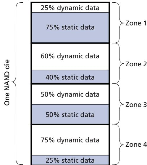
Even though static wear leveling helps ensure equal block use within each zone if the controller treats each zone separately, different zones might receive different levels of use. As such, one zone is likely to wear out before another, which would cause the die to wear out prematurely.
