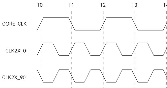
Figure 4 on page 4 shows the alignment of the CORE\_CLK with the DRAM clock. Each clock is shown with the related reference point to the DRAM signals. The phase between the CORE\_CLK and the DRAM clock can be changed if there is a delay line or a DLL that can be used to change this relationship.
