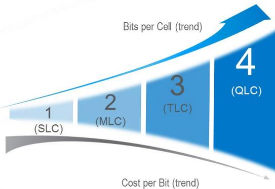
**Figure 3 – NAND Bit Density by Generation**
