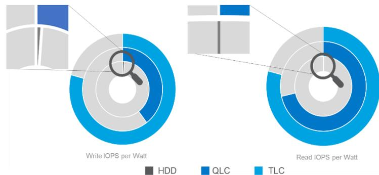
**Figure 3: IOPS per Watt Advantages of SSDs**
