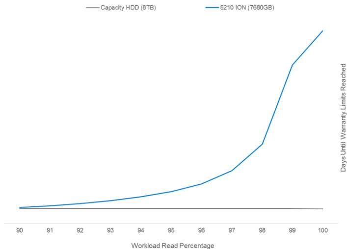
**Figure 5: Days until Warranty Limits Are Reached for Large-Block, Sequential Workloads**
