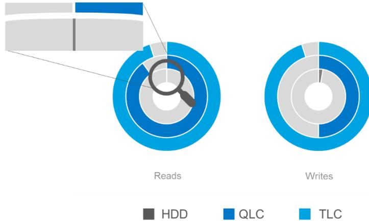
**Figure 1: Performance (IOPS) Comparison of QLC SSDs vs. SATA HDDs and TLC SSDs**
