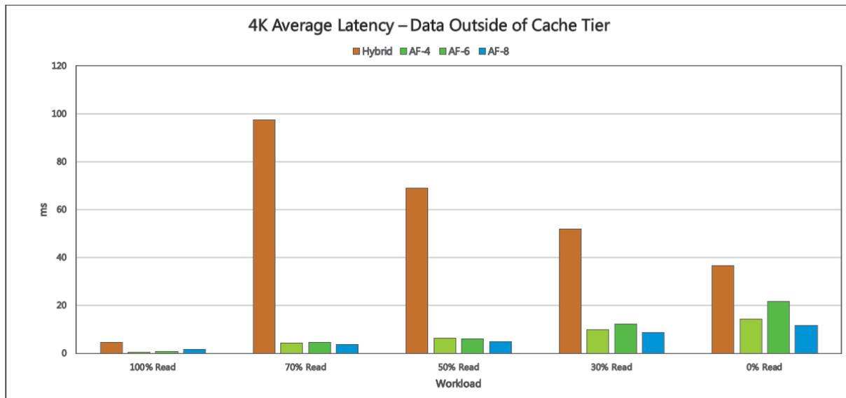
**Figure 3: HCI Bench 4K Average Latency (data outside of cache) by Workload and Node Configuration** (lower is better)
