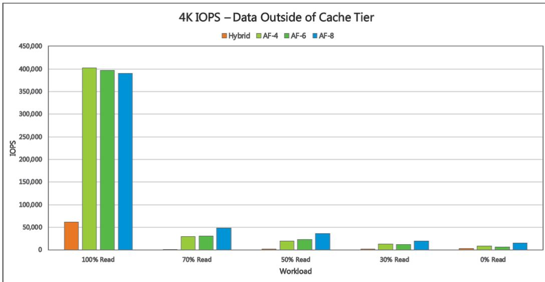
**Figure 2: HCIBench 4K IOPS (data outside of cache) by Workload and Node Configuration (taller is better)**
