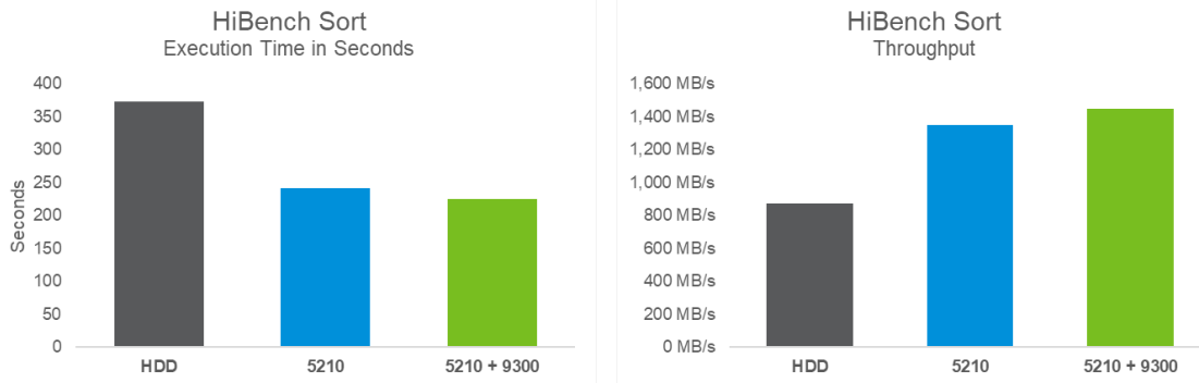
Figures 5a-5b: HiBench Sort Results: Execution Time (Shorter is Better) and Throughput (Taller is Better)
