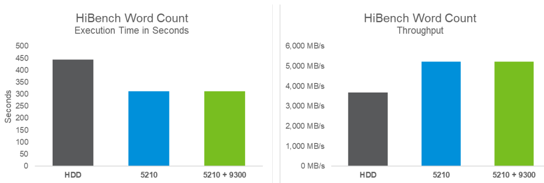
Figures 6a-6b: HiBench WordCount Results: Execution Time (Shorter is Better) and Throughput (Taller is Better)
