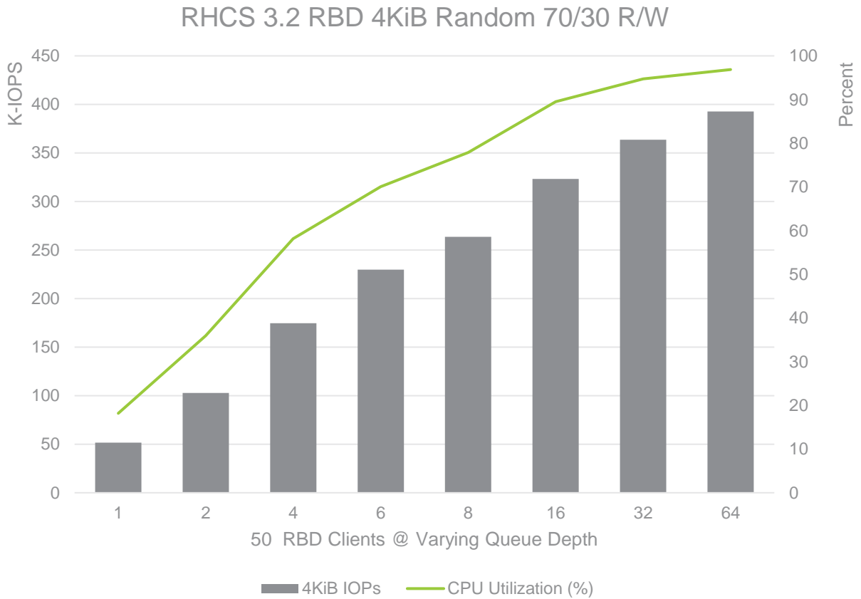
Figure 14: 4KB Random 70/30 R/W IOPS vs. CPU Utilization
