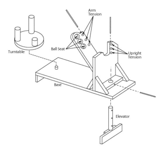
Your first task or problem to solve is to find the combinations on the catapult that will result in shooting a ball the greatest distance. The catapults have five components and three levels of each that affect the distance the ball is thrown, which is also the response variable.
