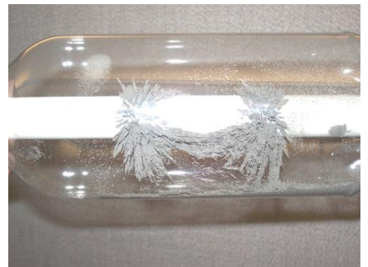
Iron filings attracted to the magnetic field in the tube viewer
